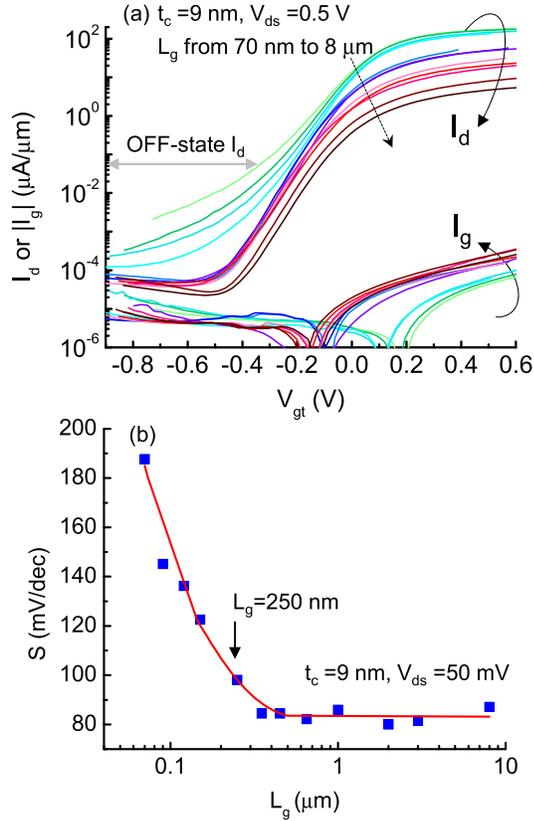
Fig. 2. (a)  $I_d$  and  $I_g$  versus  $V_{gt}$  for devices with  $L_g$  of 70, 90, 120, 150, 250, 350, 450, and 650 nm, and 1, 2, 3, and 8  $\mu\text{m}$  (color from light green to black). The transistor is biased in saturation with drain bias of 0.5 V. The  $x$ -axis is  $V_{gt} = V_{gs} - V_t$  where  $V_t$  is defined in the text. (b) Minimum subthreshold swing ( $V_{ds} = 50$  mV) as a function of  $L_g$ . For both figures,  $t_c = 9$  nm.
