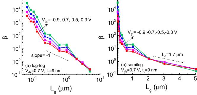
Fig. 4. Bipolar gain  $\beta$  as a function of  $L_g$  from 70 nm to 5  $\mu\text{m}$  at  $V_{ds} = 0.7$  V in log–log (left) and semilog scale (right). Different values of  $V_{gt}$  are given.
