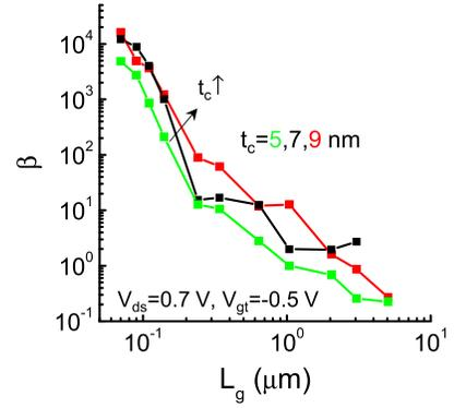
Fig. 5. Bipolar gain  $\beta$  as a function of  $L_g$  for  $L_g$  from 70 nm to 5  $\mu\text{m}$  at  $V_{gt} = -0.5$  V and  $V_{ds} = 0.7$  V. Channel thickness is varying.
