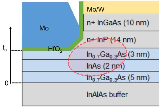
**Fig. 1.** Cross-sectional schematic of the InGaAs MOSFET studied in this paper. The gate edge of the device on the drain side is depicted. The heterostructure is specified with the layer thickness in parenthesis. Unless indicated, the ternary semiconductor compositions are lattice matched to InP. The region where BTBT takes place is colored in red.
