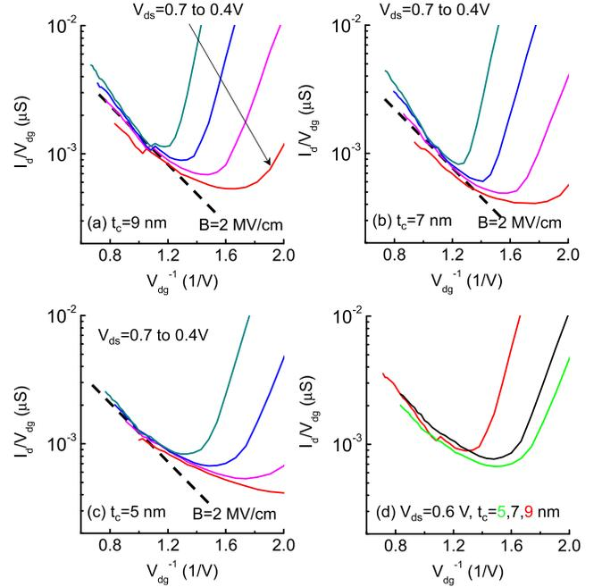
Fig. 3. Semilogarithmic plot based on (2) for  $L_g = 8$   $\mu\text{m}$  devices with (a)  $t_c = 9$  nm, (b)  $t_c = 7$  nm, and (c)  $t_c = 5$  nm. The data are extracted from the  $I_d$ - $V_{\text{gs}}$  measurement for  $V_{\text{ds}}$  from 0.4 to 0.7 V. The dashed line indicates the case when  $B$  is 2 MV/cm in (2). (d) Semilogarithmic plot based on (2) for varying  $t_c$  from 5 to 9 nm and at the fixed  $V_{\text{ds}}$  of 0.6 V. The lines overlap at high  $V_{\text{dg}}$ .
